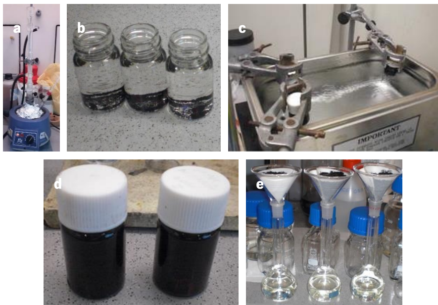
Figure 11: f-GNRs or f-GFs production illustration: (a) functionalization reaction of MWNTs or EG to obtain f-MWNTs or f-EG, respectively, (b) mixture of f-MWNTs or f-EG with ethanol, (c) sonication of f-MWNTs or f-EG solutions, (d) resultant solution after sonication containing f-GNRs or f-GFs, (e) gravity filtration of the solutions in (d)
