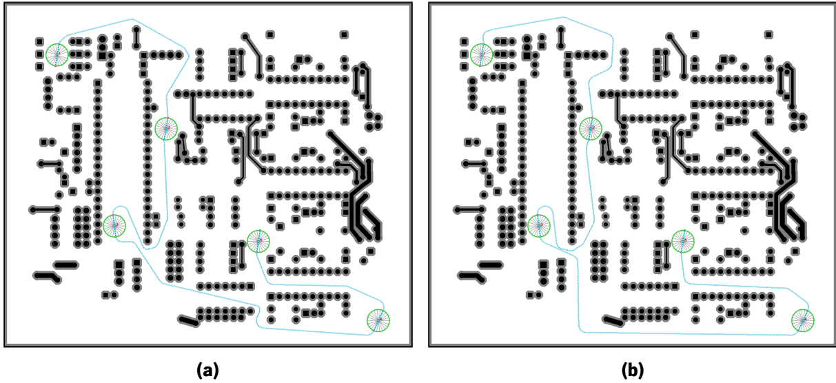
Figure 4.16: Comparison of path created by different values of PR (Penalty Radius). The results shown in (a) uses PR=1 and in (b) the PR's value is 5. For both tests the search parameters were PW=2.5, wG=0.85, wH=1.0 and \Delta=3 .
