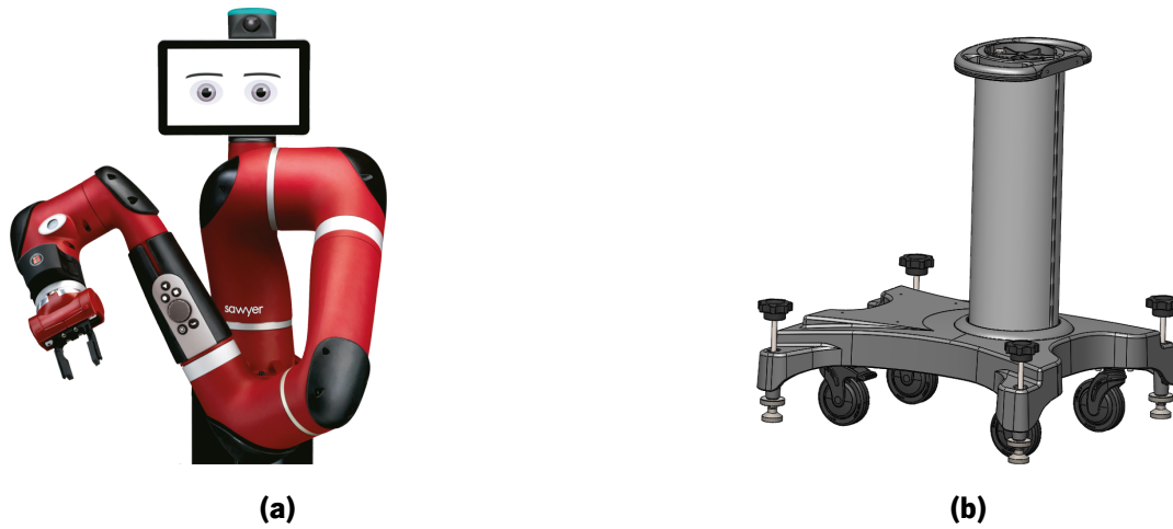
Figure 3.3: Sawyer robotic system: (a) Sawyer's robotic arm 5 and (b) its mobile pedestal 6 .
