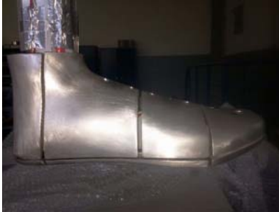
FIGURE 1. Final foot assembly with the 7 aluminium segments.
