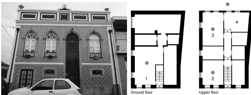
Figure 2. (left) External view; (right) Floor plans showing the position of measuring instruments (1—living room; 2—bedroom; 3—dining room; 4—kitchen).
