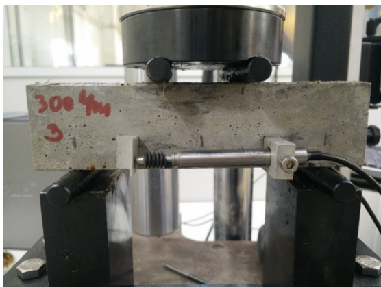
Fig. 2 Four-point bending test configuration and positioning of the LVDT on the lateral surface of the prism.
