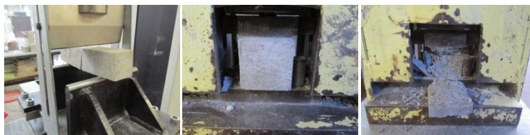
Figure 3.23 – Flexural and compressive strength tests
