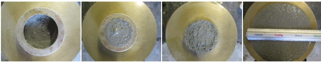
Figure 3.20 – Flow table test
