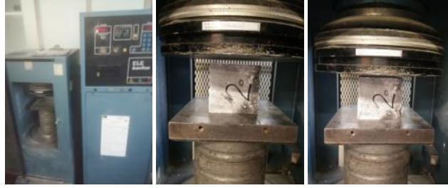
Figure 3. 28 – Compressive strength test.
