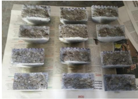
Figure 5.9 – Concrete samples after the migration chloride test
