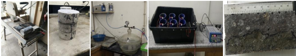
Figure 3.29 – Chloride migration test apparatus.
