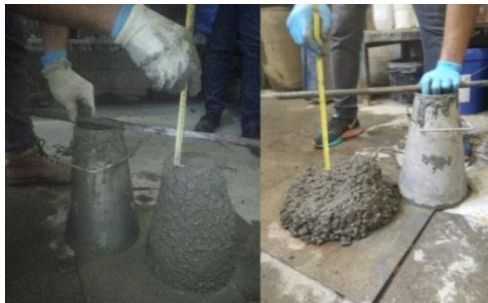
Figure 5.1 – Slump test of the reference mix (left side) and of CFA45BFA5 (right side)
