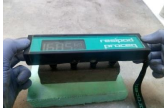
Figure 3.22 - Electric resistivity measurement
