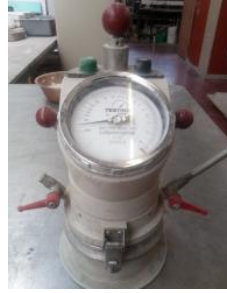
Figure 3.21 – Test apparatus showing the metal vessel and cover assembly
