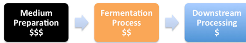
Fig. 1 The three main stages of the production process contributing for the final production cost, in decreasing cost order
