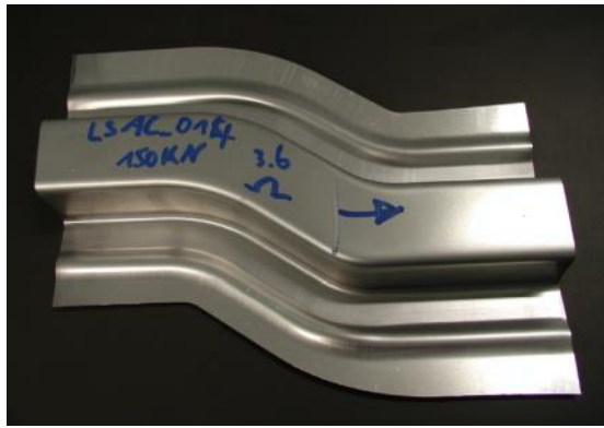
Fig. 2.1 – S-Rail topology after the drawing operation (intermediate state) for the case of smooth beads [17].
