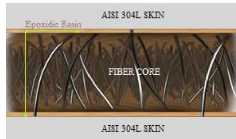
Fig. 5.2 – Scheme of the Hybrix micro-sandwich sheet material, comprising two stainless steel layers and an intermediate composite core (metallic/polymeric fibers embedded in an epoxy resin).
