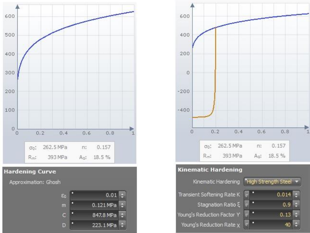
Fig. 3.5 – Mechanical and constitutive parameters of the yield criteria and hardening models used in the variability study [63].
