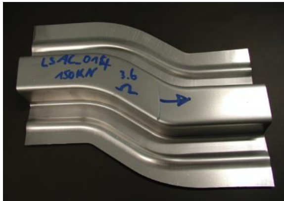
Fig. 3.1 – S-Rail topology after the drawing operation (intermediate state) for the case of smooth beads [63].
