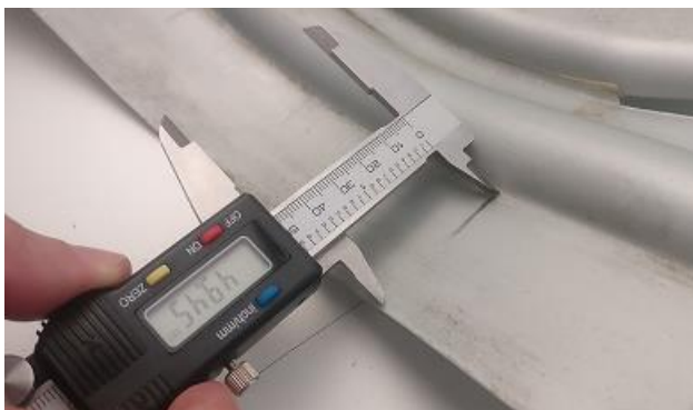
Fig. 6.8 – Experimental measurements of the y-distances in cross sections defined in the study and marked in the part.
