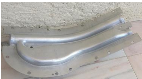
Fig. 6.1 – Stamped Prototype of an aluminium automotive fuel filling system designed by Sodecia.
