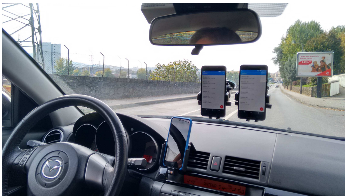
Figure 9: Equipment setup for the first run, a symmetric configuration with two similar smartphones running the same software versions, mounted on similar car mounts in similar positions and location, inside a vehicle
