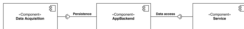
(b) High-level component diagram, detailing the relationships between Data Acquisition and other components of the system
