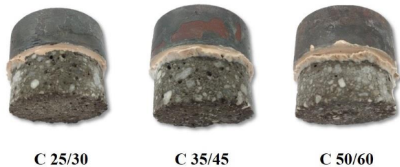
Figure 5. Visual determination of the type of failure (pull-off test).
