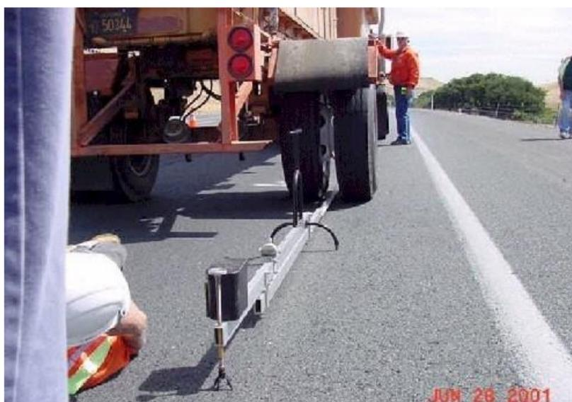
Figura 9: Ensaio com viga *Benkelman* (Pavement Interactive, 2018)
