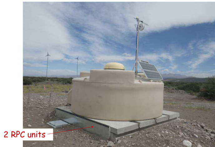
Figure 6.1 – Picture of TdF’s station. Below the tank there are 2 RPC units, one on top of the other. [74]
