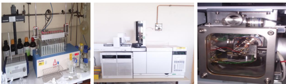
Figure 12 - a) Test tubes, b) Exterior of the Equipment used in the laboratory to quantify 5-FU (Chromatograph), c) Inside.
