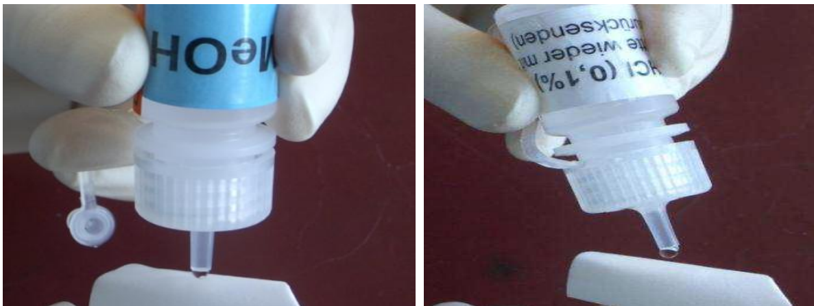
Figure 5 - Fixative application (MeOH) and (HCl) to the paper filter (reproduced from Schierl, 2009).
