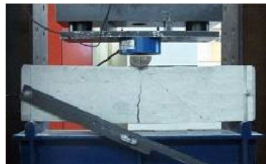
Figure 6 – Bending test of concrete beams reinforced by braided reinforced composite rods
