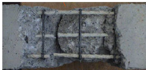
Figure 7 – Beam produced with braided reinforced composite rods after testing
