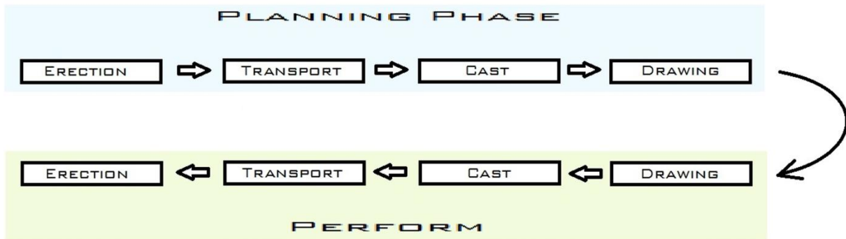
Figure 1: The planning and perform process of precast.
