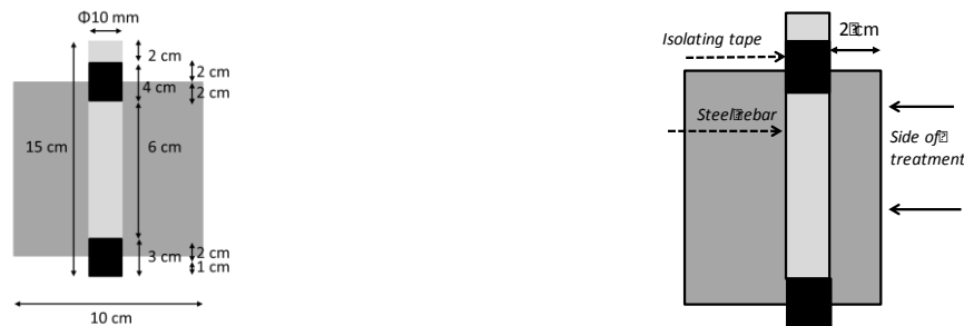
Figure 1: Left – Concrete sample dimensions after casting. Right – Concrete samples prepared for testing.
