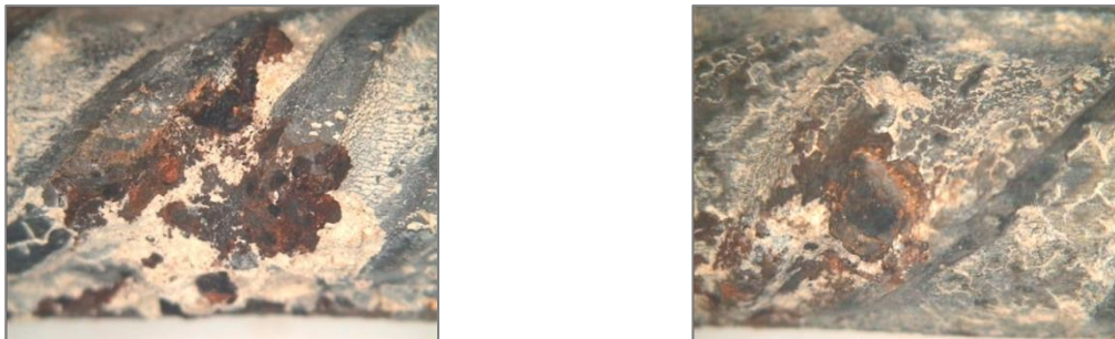
Figure 5: Images from the optical microscope of corrosion points at the end of the test. Left: sample without surface treatment after. Right: sample treated with the corrosion inhibitor.
