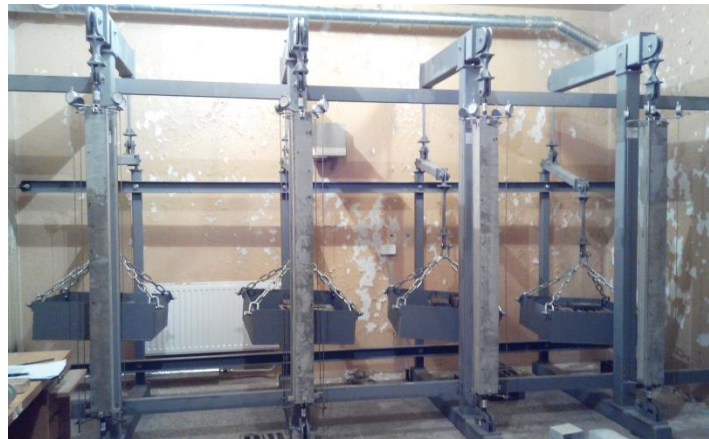
Figure 2: Photograph of ongoing creep test.
