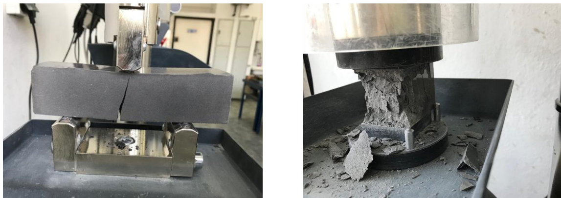
Figure 1: Left: an example of the flexural failure, Right: an example of compression failure.
