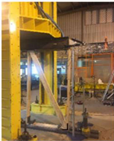
Figure 7: Diagonal bracing walls in test.
