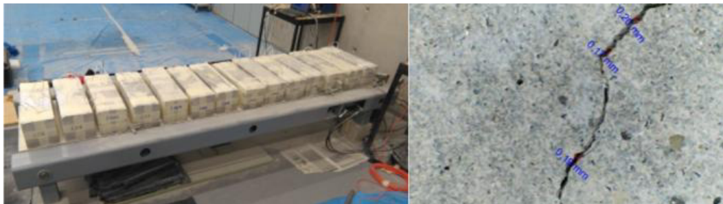
Figure 4: Load blocks (left) and crack at midspan after application of the load blocks (right).
