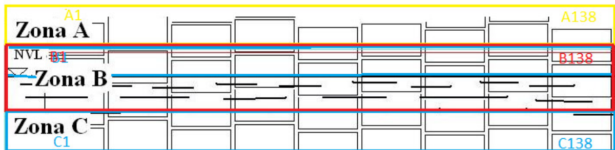
Figure 1: Zoning of slabs (in vertical direction): zone A – above the changeable water level; zone B – at changeable water level (above or below NWL); zone C – zone under water (below NWL).
