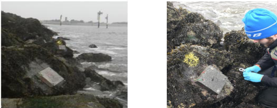
Figure 1: Concrete tiles installation and deployment.
