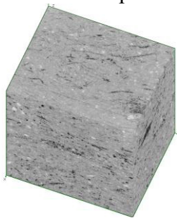
Figure 1. Three-dimensional projection of the 4 \times 4 \times 4 mm piece of specimen 'B'. Some ca. 1 mm long fibres are visible in the bulk of the material.
