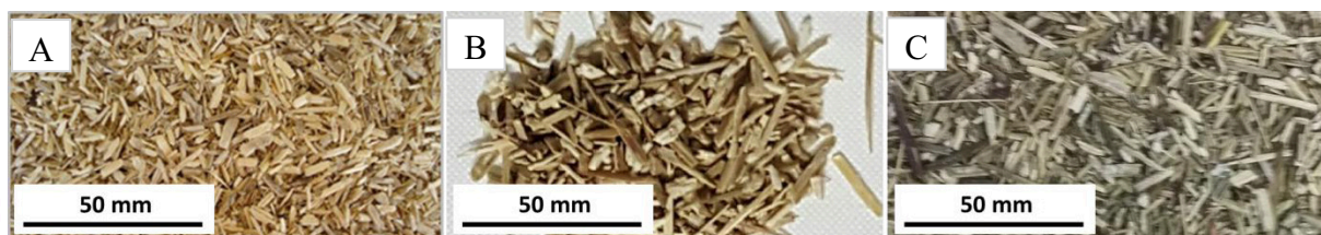
Figure 1: Photographs of the three studied bio-aggregates: hemp shives (A), corn (B) and sunflower (C) bark particles
