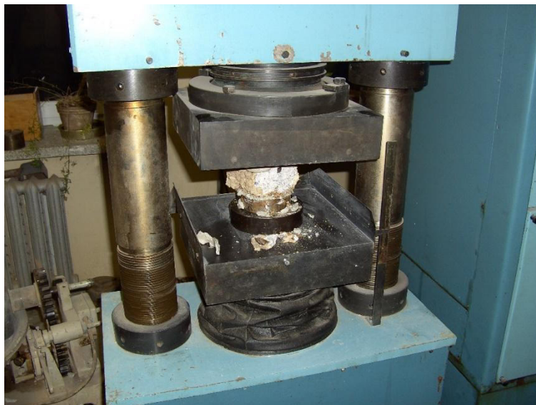
Figure 2: The sample in hydraulic press MC-1000
