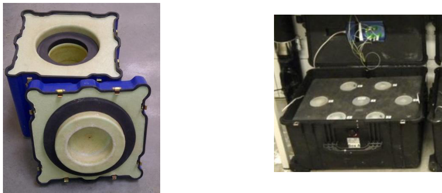
Figure 1: the QAB calibrated calorimeter used on concrete (left) and the non-calibrated calorimeter used on small sample (right).
