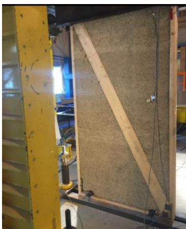
Figure 9: Diagonal bracing hemp walls in test.
