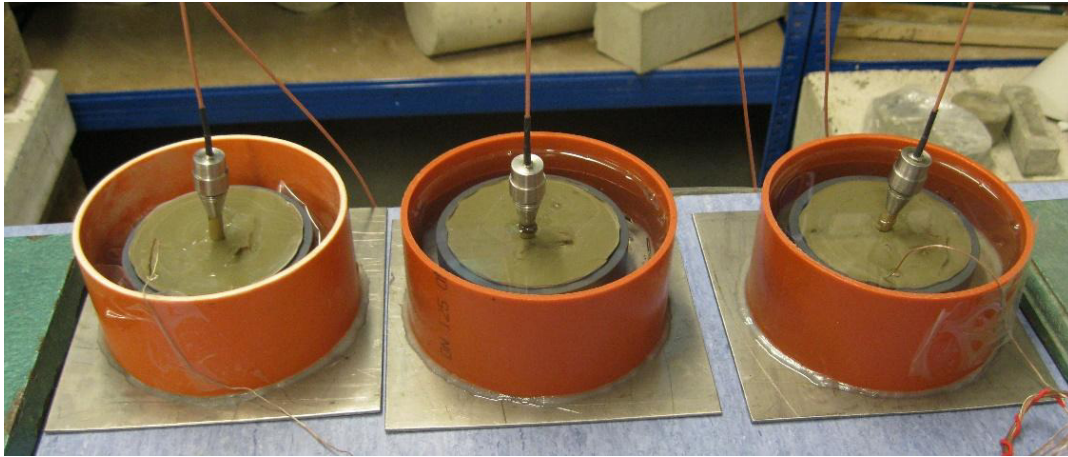
Fig. 2 Photo of placement of the AE sensors.
