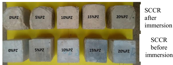
Figure 5: SCCR specimens degradation before and after immersion in 5%Na 2 SO 4 solution.
