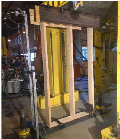
Figure 3: Empty vertical stud frame in test.
