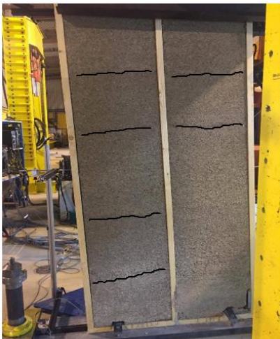
Figure 5: Vertical stud hemp wall in test.
