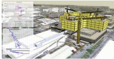
Figura 4 – Interface BIM-CS
