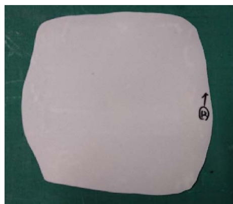
Figure 2. Thermo-responsive TSG/LLDPE/CaCO 3 film.
