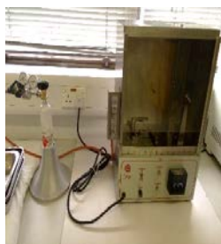
(b) Flame resistance tester (Model: TC-45 220V 50HZ)
