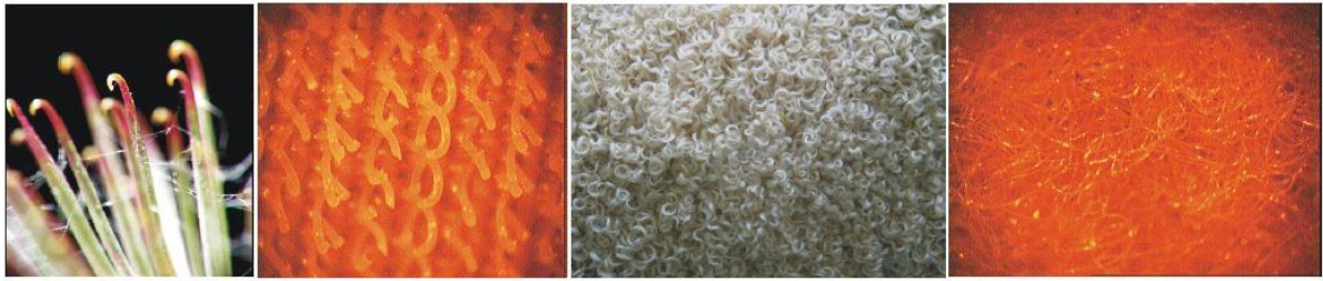
Figure 4, the inspiration to Velcro and its technological imitation. From left to right: The hooks of the burdock seed and the artificial loops. The wool from a sheep and the artificial loops. (Wilhelm Barthlott and Neinhuis, 1997).
