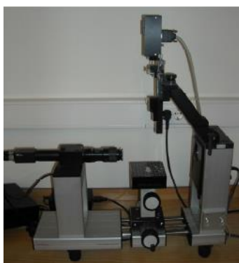
Figura 31 - Goniómetro OCA 20, DataPhysics Instruments GmgH, Filderstadt.
