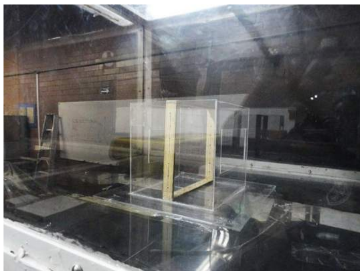
Figure 1. 3D Physical scale model 1 showing section frame with Thin wires for visualization technique
