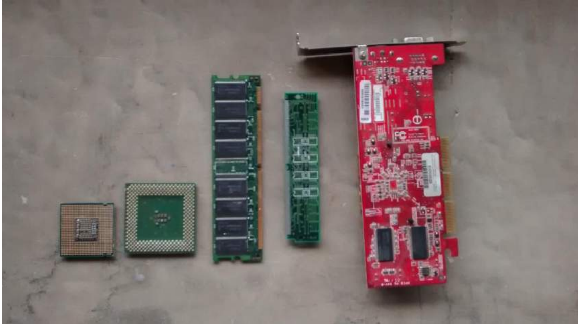
Figure 1 – Boards in different sizes. From left to right: processor, processor, RAM, RAM and video card.
