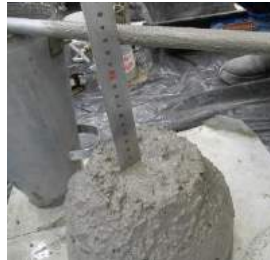
Figure 4. Determination of consistency through Slump Test.
