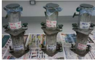
Figure 5. Samples in placeholder in the laboratory, waiting to be extracted from the mold.
