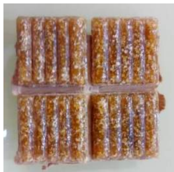
Figure 2 –Recycled glass tile in dimensions 2,5x2,5cm.
