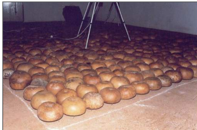
Figure 4: raised pieces with opening down put together in the reverberation chamber
