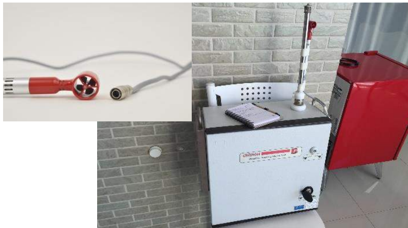
Figure 2. Meteorological sensor used on monitoring the balconies
