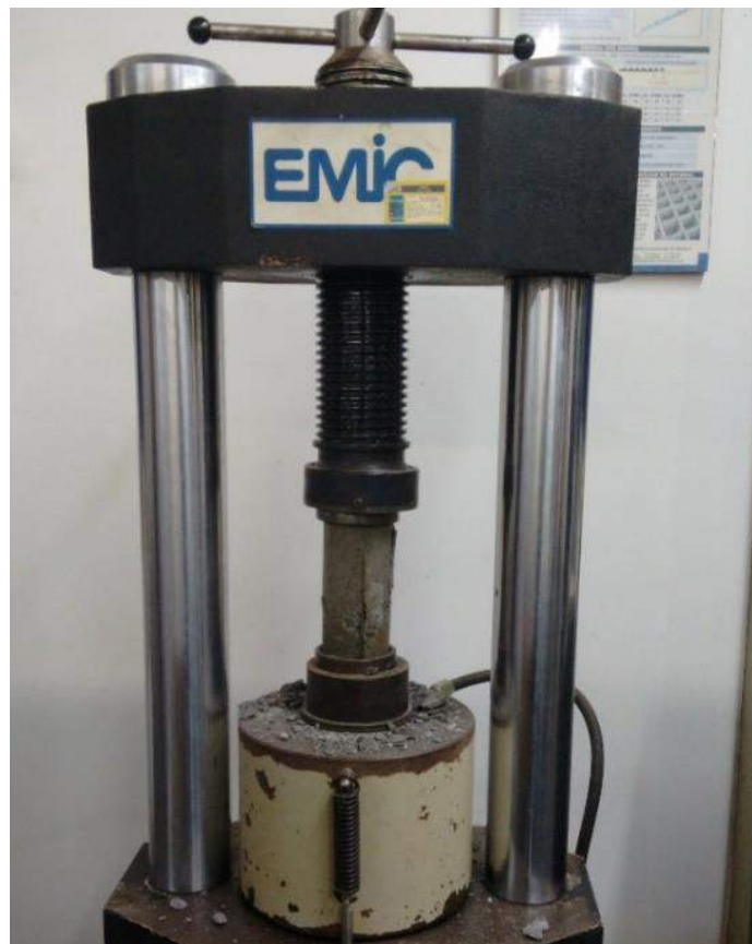
Figure 1. Axial compression strength test. Source: Authors, 2016
