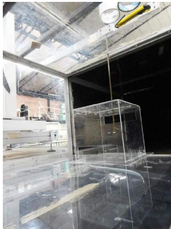
Figure 3. 3D Physical scale model N2 showing section frame with thin wires for visualization technique and hot wire anemometer for pressure and wind speed measuring
