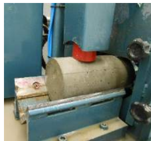
Figure 7. Sample being rectified, to prepare de base.
