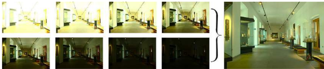
Figure 3. Sequence of photographs with different exposure ranges with final image in HDR (source: own preparation).
