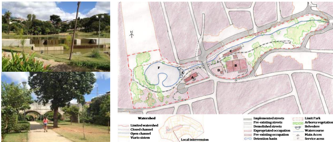
Figure 8 and 9. (Left) Spillway, detention basin and way within the park. Source: Bueno, 2016
