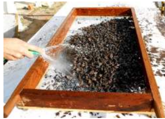
Figure 2. Coarse aggregate being washed
