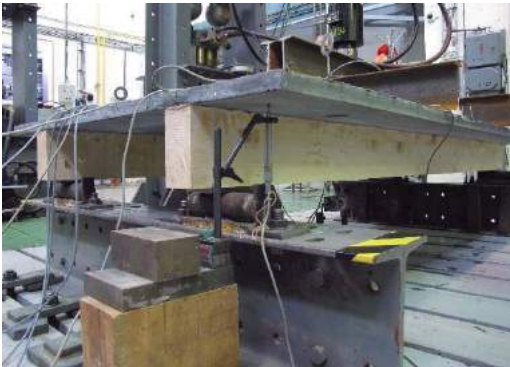
Figure 7. Load test of composite floor element at CTU in Prague laboratories. Figure 8. Life Cycle Tower One, Dornbirn (source: H. Kaufmann).
