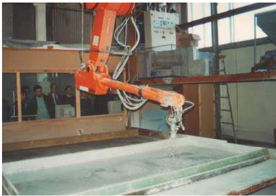
Figure 3. Examples of a robot in the casting process and a possible layout of an assembly line (Pastor et al. , 2005)
