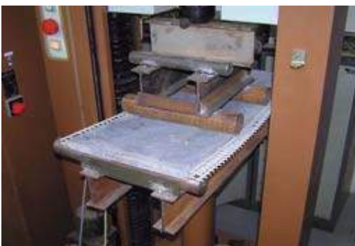
Figure 9. Testing of TRC thin plate element (CTU in Prague laboratory). Figure 10. Prototype of façade element from white TRC (produced at SKANSKA CZ company).
