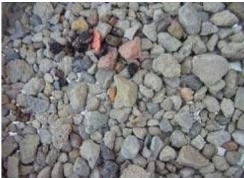
Figure 3. Recycled concrete from demolition
