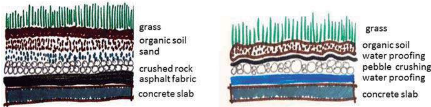
Figure 1. Schematic layers of analyzed green roofs in a big and medium city respectively.
