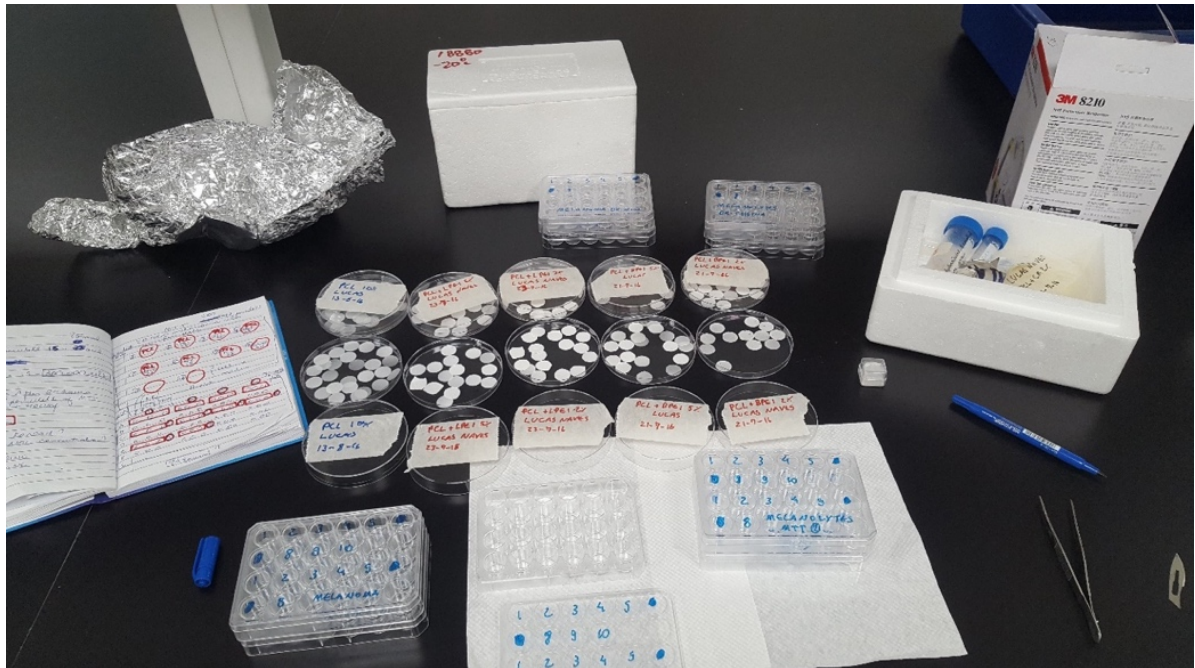
Figure 3-2 Labeling the electrospun mats for biological tests. of PCL, PCL_2LPEI, PCL_5LPEI, PCL_2BPEI, PCL_5BPEI. Abbreviations: PCL: -poly( \epsilon -caprolactone), PCL_2LPEI: poly( \epsilon -caprolactone) blended with 2% of linear Polyethyleneimine, PCL_5LPEI: poly( \epsilon -caprolactone) blended with 5% of linear polyethyleneimine, PCL_2BPEI: poly- ( \epsilon -caprolactone) blended with 2% of branched Polyethyleneimine, PCL_5BPEI: poly( \epsilon -caprolactone) blended with 5% of branched Polyethyleneimine, TCP: tissue culture plate.
