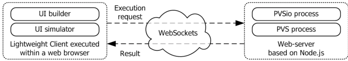
Figure 5: Diagram of the client-server communication mechanism in PVSio-Web, extracted from [Oladimeji et al. (2013)].
