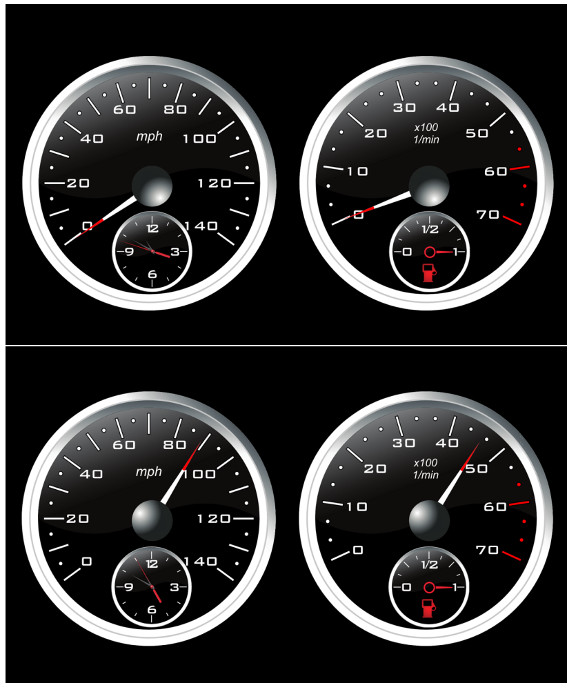
Figure 49: Second car dashboard prototype in its initial state (top) and after accelerating the car (bottom).
