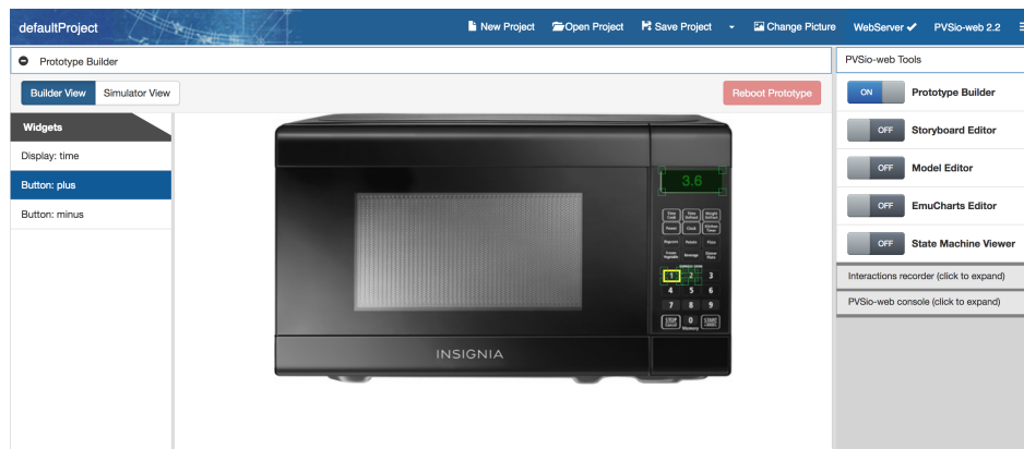
Figure 7: Example of the construction of a simple prototype of a microwave, with a time display and two buttons (“plus” button currently selected).
