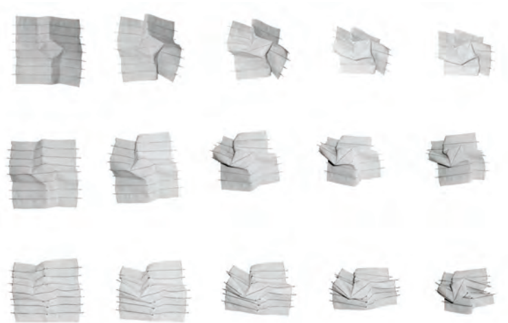
Figure 42. Squaretwist samples during thermal activation (1st row 0,2 mm wire sample; 2nd 0,3 mm and 3rd 0,5 mm).
