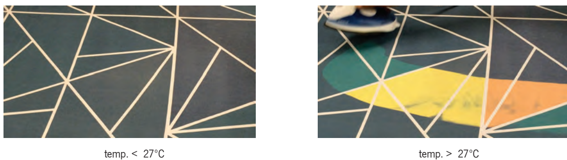
Figure 28. Study prototype section, below and above 27°C.
