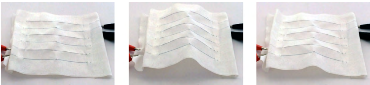
Figure 55. Sample deformed (left); 1st Actuator group activated (centre) and 2nd Actuator group activated (right).
