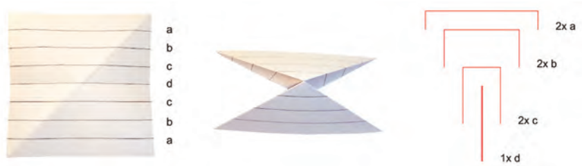
Figure 38. Waterbomb model open and close (left and centre); SMA shapes (right).
