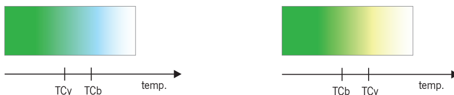
Figure 4. Example of gradual colour change with TC pigments combination.
