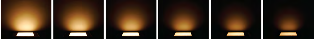
Figure 33. Pile-up of textiles from one to six layers (left to right, respectively).
