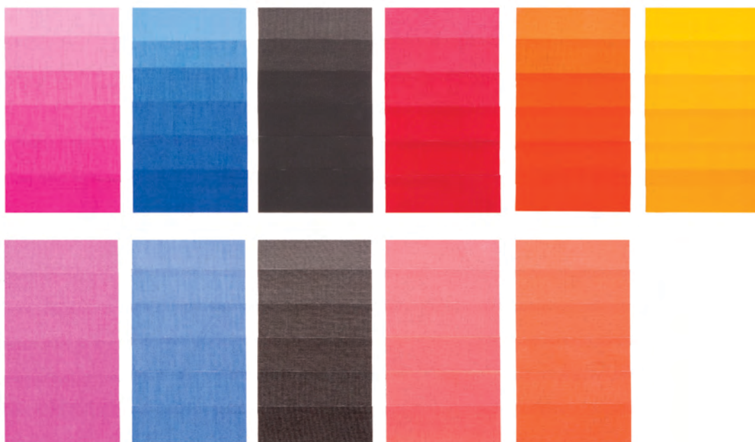
Figure 17. Samples with different concentrations of conventional pigments (1 st row) and TC pigments (2 nd row).
