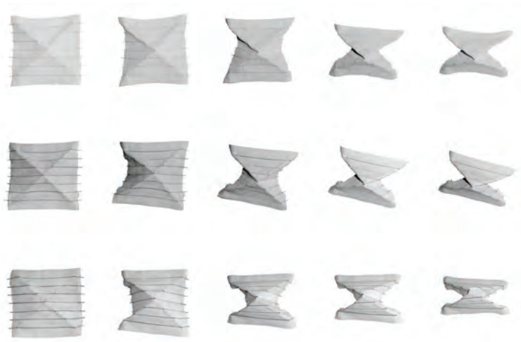
Figure 41. Waterbomb samples during thermal activation (1st row 0,2 mm wire sample, 2nd 0,3 mm and 3rd 0,5 mm).
