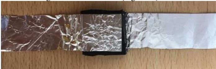
Figure 10. Sensor with conductive silicone and aluminium foil
