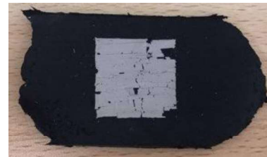
Figure 7. Sample with conductive silicone and PE 825 conductive ink
