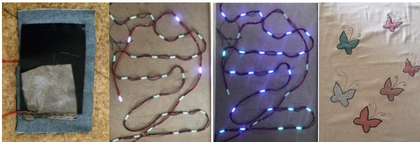
Fig. 3. From left to right a) Force sensor, b) Illuminated circuit activated by the sound sensor, c) Illuminated circuit activated by the force sensor, d) Front view of the panel
