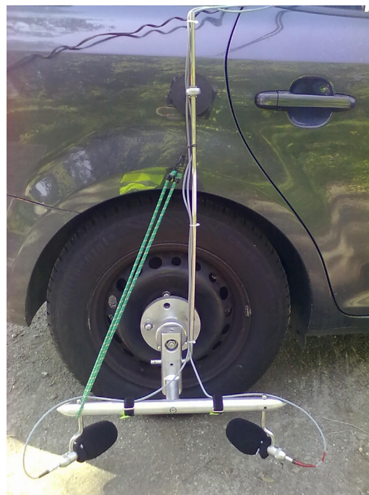
Fig. 4. Microphones mounted in the test tyre.
