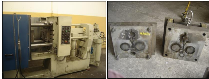
Figure 1. 180 tons of clamping force cold chamber die casting machine (left) and a casting die (right).
