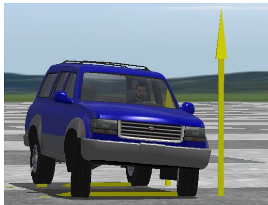
Fig 8. Fishhook test: visualization of lift-off.
