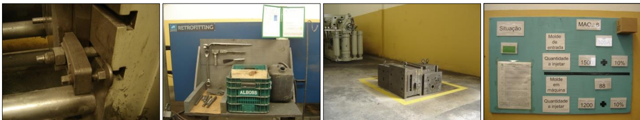
Figure 6. Die clamp with leveler, tools panel, dies island and setup panel, respectively.
