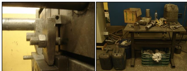
Figure 3. Die clamp with shim (left) and the old tools table (right).
