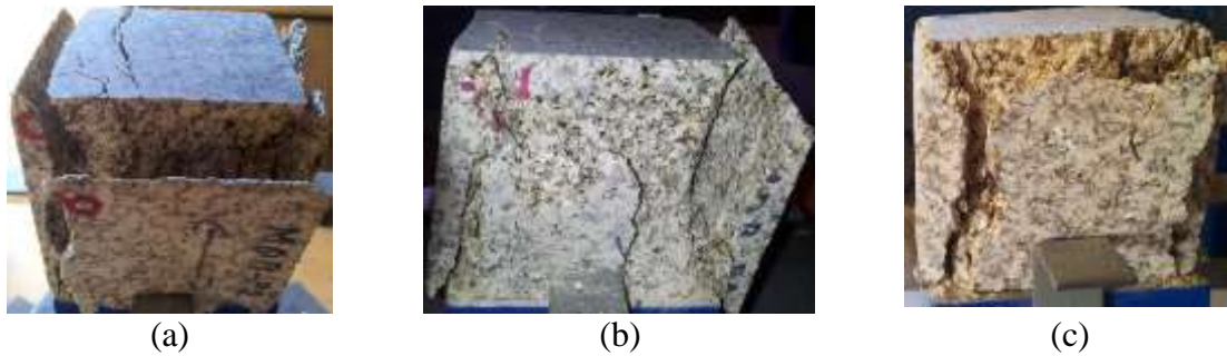
Figure 27. Typical failure modes for uniaxial compressive test before freeze–thaw cycles: (a) MDB samples, (b) PTM samples and (c) FT samples
