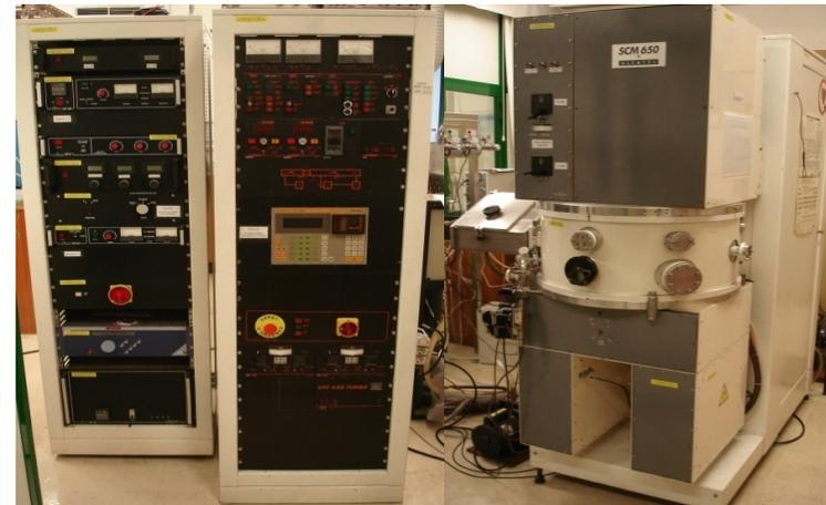
**Thin film deposition systems: Magnetron Sputtering – DC and pulsed DC mode**
