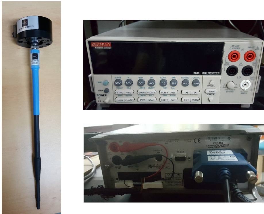
Figure 49 - The SAR probe is on the left and on the right, the modified Keithley multimeter, used to perform the acquisition (front view on top and back view on the bottom).
