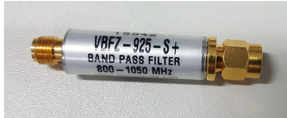
Figure 33 - Bandpass filter used in the demodulation block.
