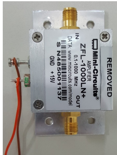
Figure 45 - Optional amplifier for the receiving block of the communication link.
