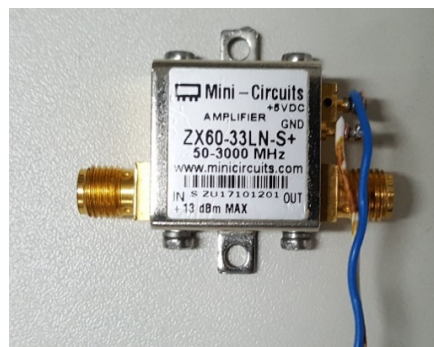
Figure 44 - Optional amplifier for the transmission block of the communication link.
