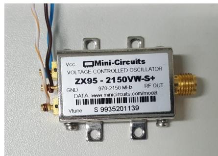
Figure 32 - VCO used as the RF source for the communication system.
