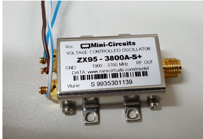
Figure 26 - VCO that was used as RF source for the WPT system.
