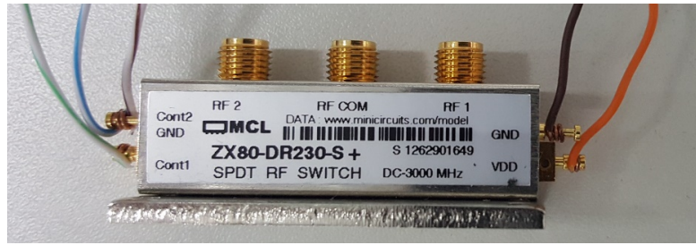
Figure 42 - RF switched used for the modulation and managing the antenna access.
