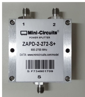
Figure 25 - Splitter used to generate two identical RF signals.
