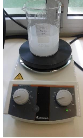
Figure 15 – Sample 2 on magnetic stirrer [1,0% MCC w.r.t. water]
