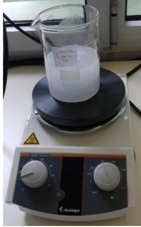
Figure 14 – Sample 1 on magnetic stirrer [0,4% MCC w.r.t. water]
