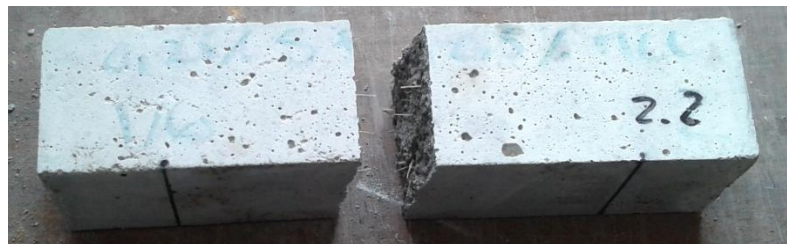
Figure 27 - Sample 2.2 after flexural testing
