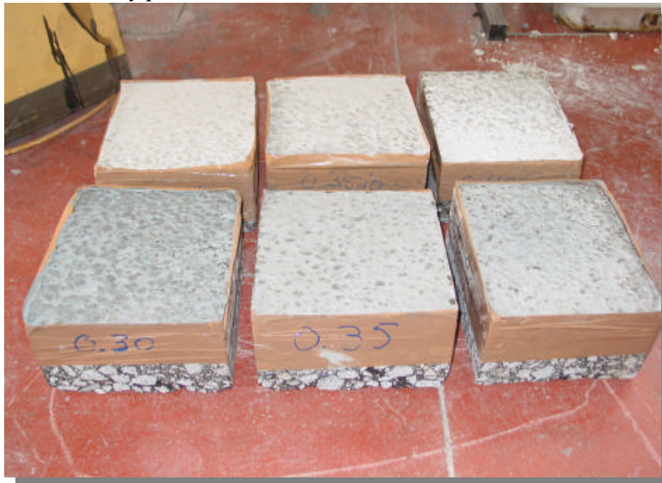
Figure 3 – Slabs filled with cement grout
