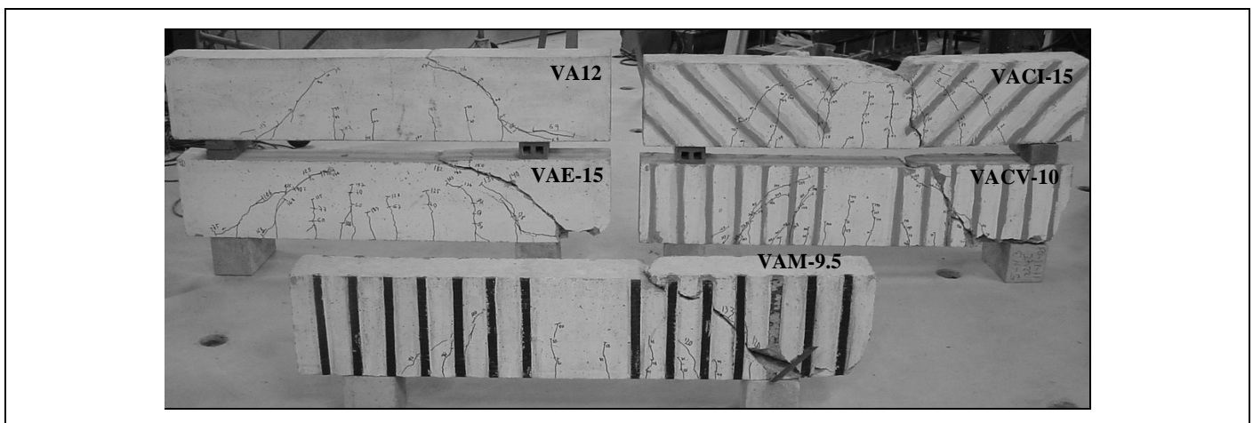
Figure 10 - Failure modes of the beams of A series with 4\phi 12 .
