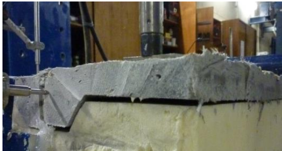
c) Slip between DHCC layer and GFRP ribs
