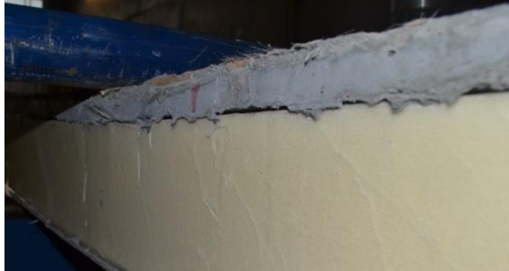
a) Loss of connection between DHCC layer and foam core
