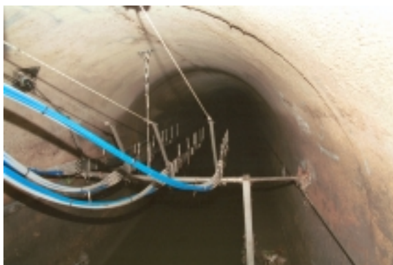
Figure 2: Orphée: the 2D sampler in the raised position
