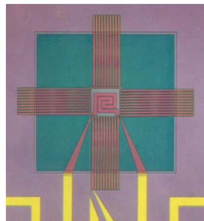
Fig. 1: Photograph of a micromachined thermopile. The nitride membrane, the silicon absorber, the self-test heater and thermocouples can be seen.
