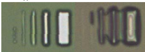
Fig. 5 Test structures for determining the minimum channel width. BCB thickness 4\mu\text{m} (left), 7\mu\text{m} (right)
