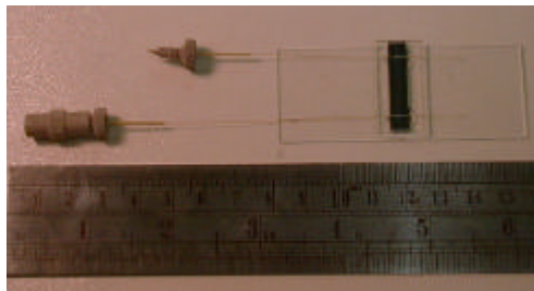
Figure 3. Polymer bonded fluidics component to a device with integrated fluidics.
