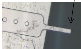
Figure 3. Photograph of a pipette nozzle 11 \mu\text{m} -wide and 2.5 \mu\text{m} -high (inner diameter: 10 x 1.5 \mu\text{m}^2 )
