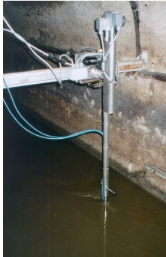
Figure 3: "Cerbère": the 2D remote-controlled device for measuring velocity fields
