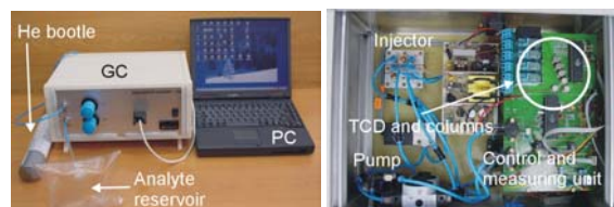
Fig. 1. The portable gas chromatograph: left - the instrument, carrier gas bottle, and PC, right - inside parts.
