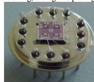
Fig. 1: View of a micro-array mounted on standard TO-8
