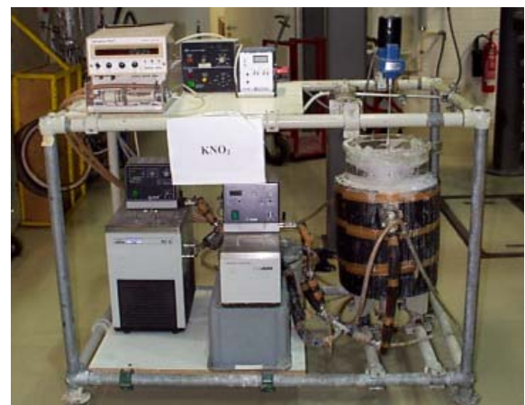
Fig. 2. experimental setup with a crystallization vessel
