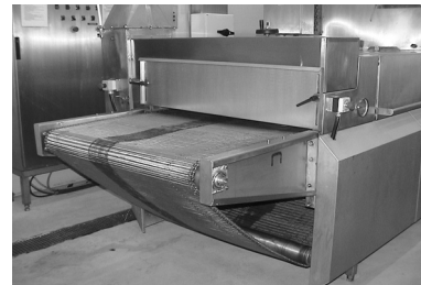
Fig. 1. The Industrial Conveyor Belt Oven used in Tests
