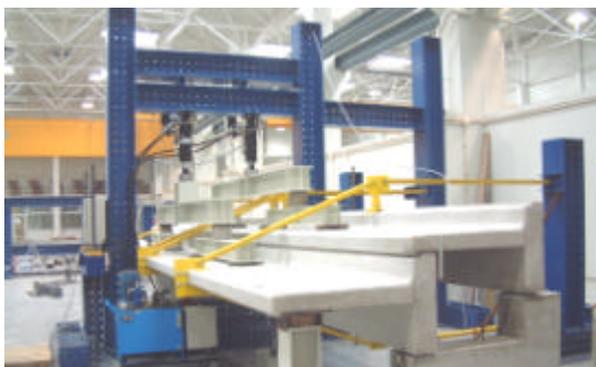
Fig. 4: Picture of the simple support bench structure
