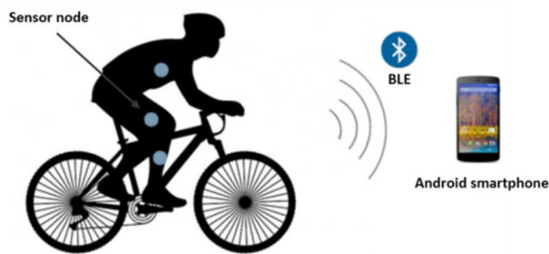
Figure 1. Architecture of the developed cycling posture monitoring system.
