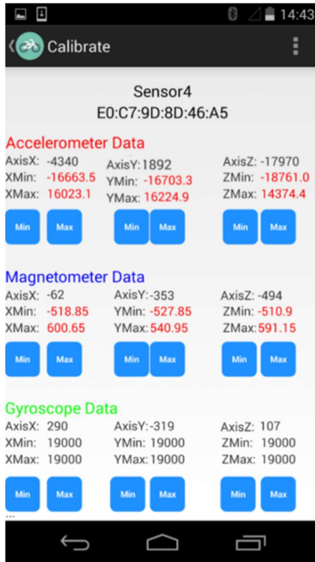
Figure 6. Sensor calibration panel of the smartphone application.
