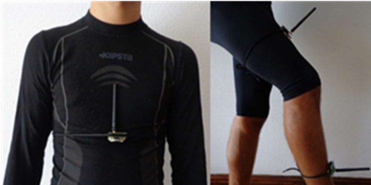
Figure 7. Sites of placement of the sensors on the athlete's body: torso (left) and leg (right).
