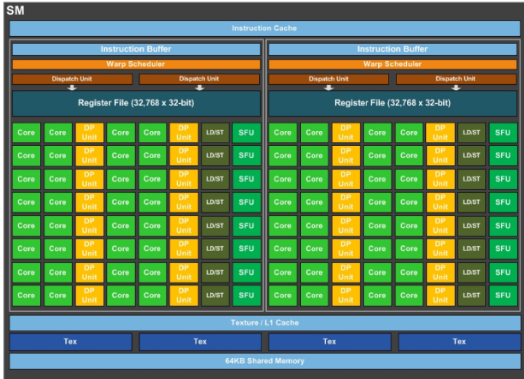
Figure 7: The Pascal GP100 Streaming Multiprocessor (from: [23])
