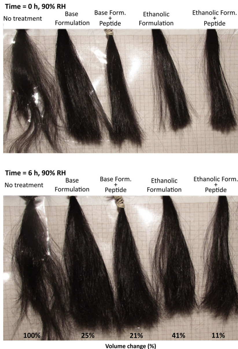
Figure 6 Images of Caucasian hair tresses at the beginning of the test (0 h) and after 6 h at 90% RH.
