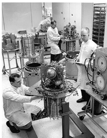
Figure 2.4 – A bacon fuel cell was chosen by NASA to provide energy for the Apollo spatial module [4].
