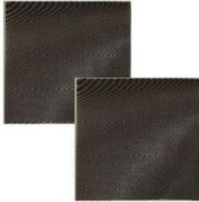
Figure 3.3 - A Nafion® membrane from Dupont.
