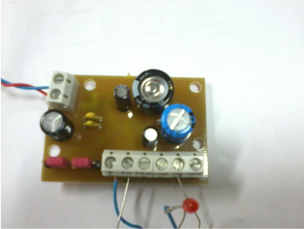
Figure 5.8 - Upper side of the designed PCB, with several capacitors and connectors
