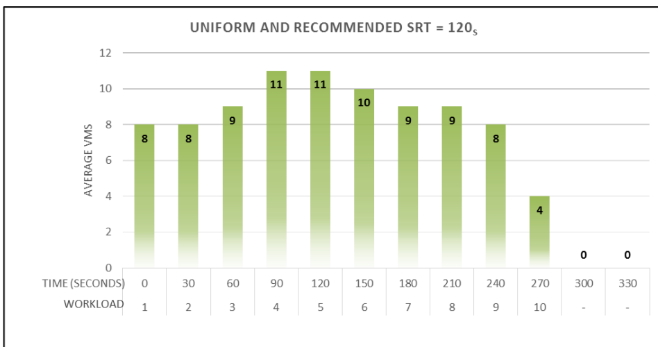
Figure 5-4. Type 1 Requests (Select-Aggregation): average virtual machines used for workloads uniformly arriving every 30 seconds for the Recommended SRTs: 80, 100 and 120 seconds.
