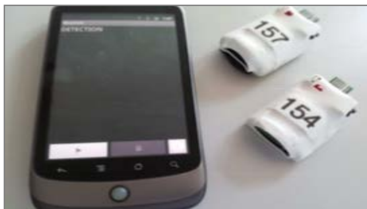
Figure 3.15 - The FOG-Assist system on a Nexus One smartphone with external accelerometers. Taken from [51].
