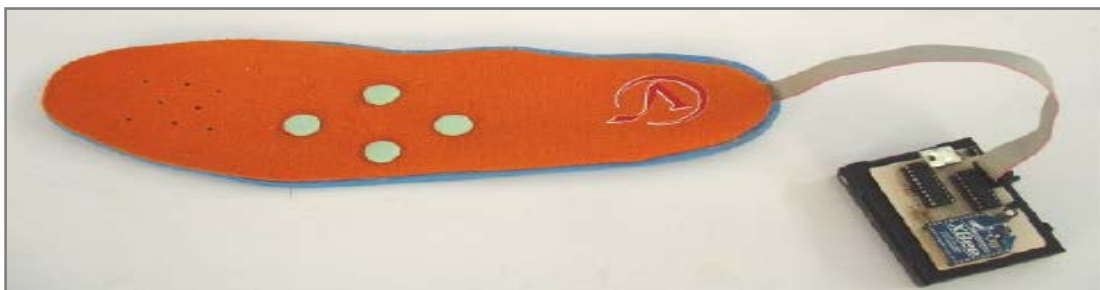
Figure 3.18 - Second prototype of shoe-integrated tactile display (4-point array of actuators). Taken from [16].
