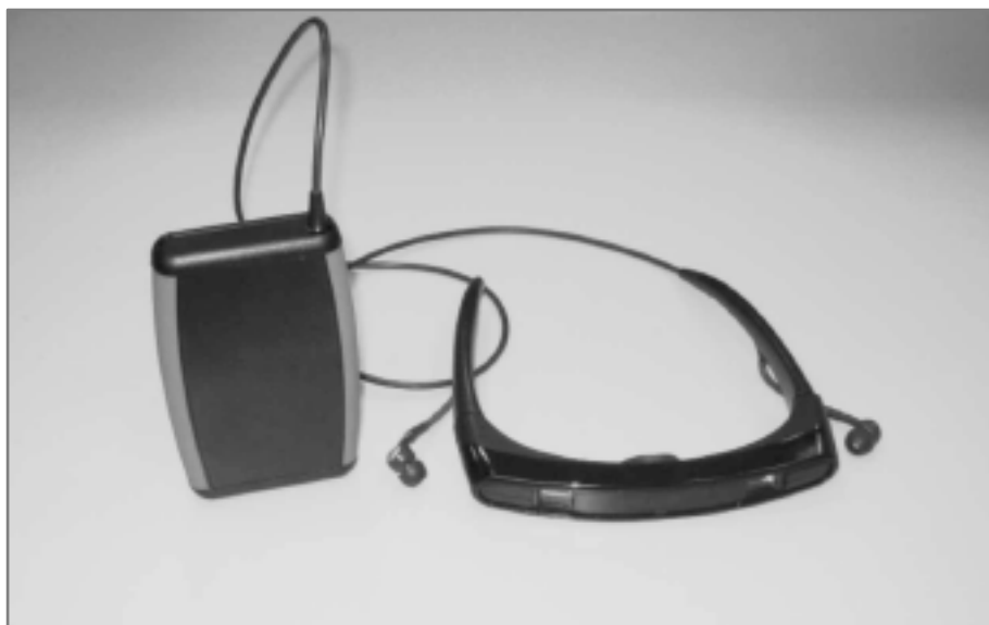
Figure 3.8 - Virtual reality goggles, containing a built-in LCD screen between the visors and earphones, attached at the belt. Taken from [49].
