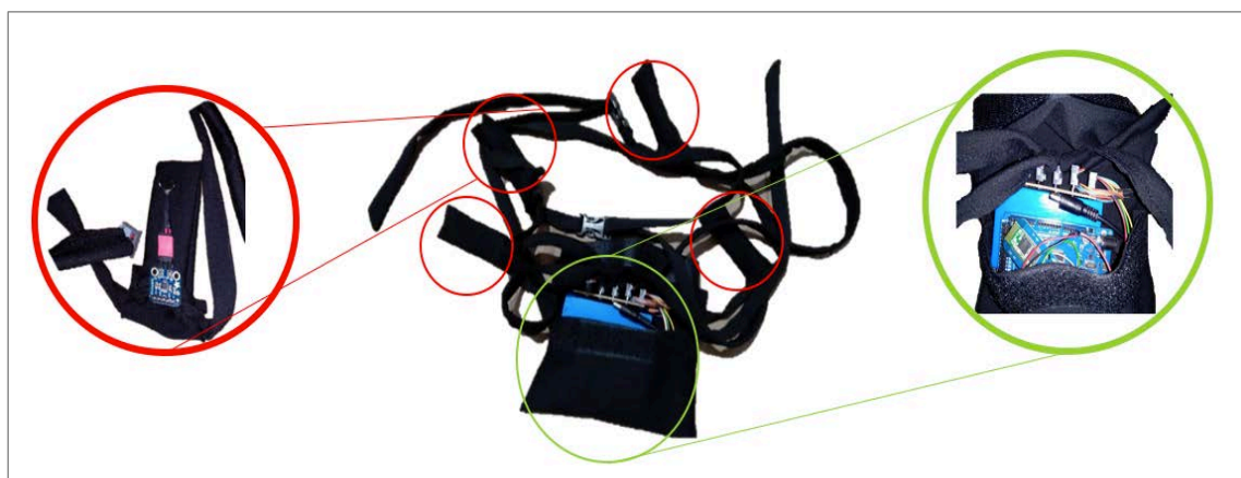
Figure 5.3 - Belt system discrimination: the processor unit, the wireless communication component and the power supply system allocated at the larger bag, demarcated at green; and the four actuation system, with the vibrotactile units, placed at the longest bags.
