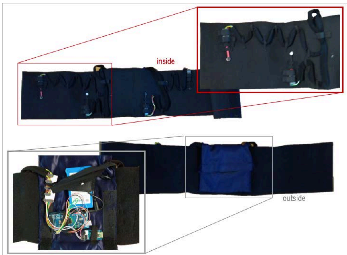
Figure 5.5 - The waistband: at top, an inside view, highlighting the vibrotactile units (demarcated at red) and in down, an outside view, emphasizing the majority electronic components (demarcated at grey).
