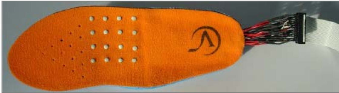
Figure 3.17 - First prototype of shoe-integrated tactile display (16-point array of actuators). Taken from [16].
