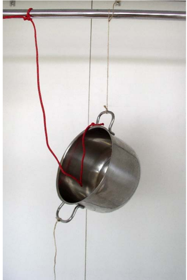
Figure 3. The pot prepared for the breaking of the string (The thicker string acts as a safety device to prevent the pot from striking the floor)
