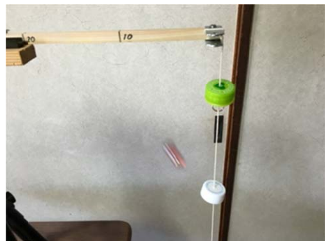
Figure 4. The apparatus to test the rule of the projectile motion (up). If we put the targets at one of positions on the parabola, the ball hits the target as (down)
