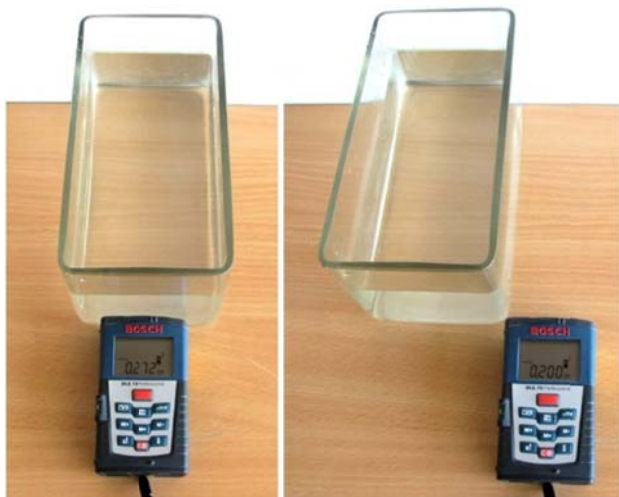
Figure 10. Principle of the measurement of the refractive index
