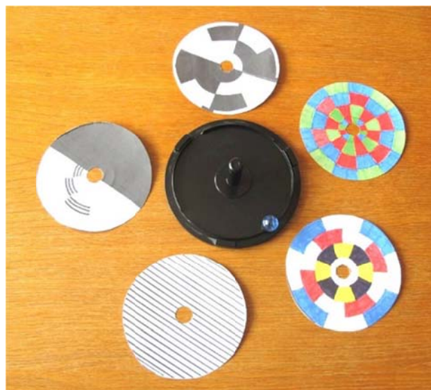
Figure 5. Mixer of colours (the marble should be glued to a bottom of it, or simply putted under the bottom)
