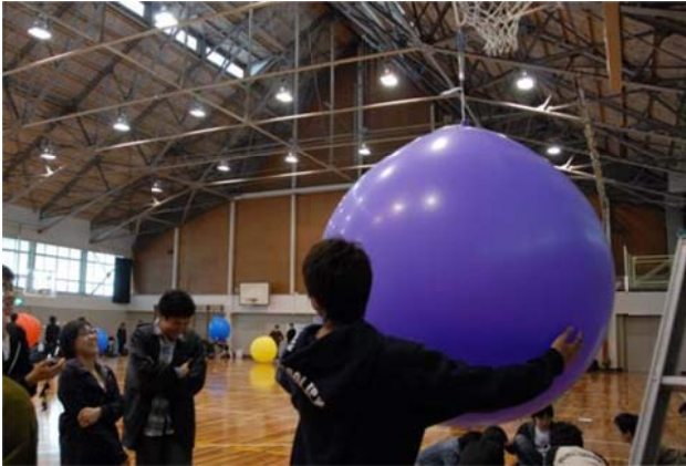
Figure 2. Students are trying to measure the mass of the air in the balloon by vibrating the balloon fixed to the spring
