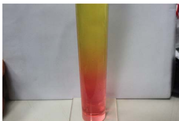
Figure 4. The second layer fills yellow liquid, which contains half saturated salt water and half clean water
