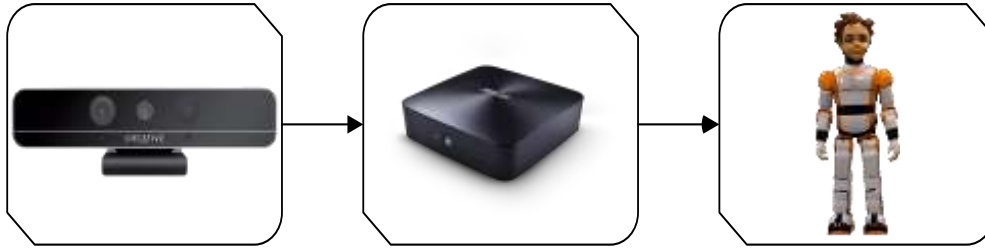
Figure 4.2-1 . Experimental setup. Starting from the left: Intel RealSense (model F200), computer and ZECA robot.
