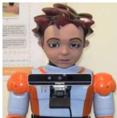
Figure 5.1.3-1 Experimental setup: ZECA and Intel RealSense.
