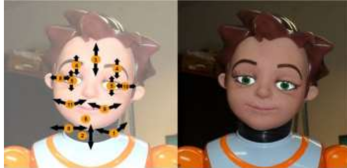
Figure 4.2.3-1 Mapping of the servo motors on the face and the neck of ZECA (Costa, 2014).
