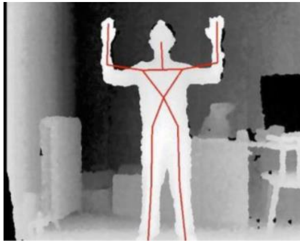
Figure 15 – Example of an approach for detection of a human skeleton 4 by using the Microsoft Kinect sensor [43].
