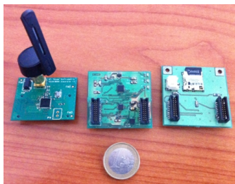
Figure 1: Sensor node prototype. The CC2530 module is shown on the left, the sensor and battery board in the middle and the SD card board on the right.
