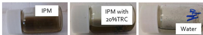
Figure 1. Visual illustration of fullerene C_{60} dispersions (0.8 mg/mL) in IPM (left), in IPM with Transcutol (20% TRC) (center) and in water (right).
