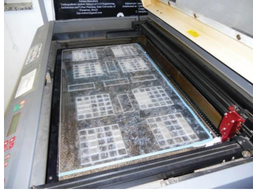
Fig. 6. Confection of the acrylic facades Prototypes by a laser cutter.
