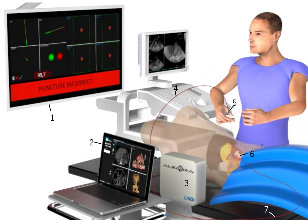
Figure 4.13. Representation of the surgical setup when using the Aurora system. The Aurora field generator (3) creates an electromagnetic working space where the needle (5) and catheter (6) can be manipulated. Both tool are wired (4 and 7) connected through the SCU to the KidneyNav software (2). The surgeon can be guided towards the anatomical target (6) using a navigation interface (1).
