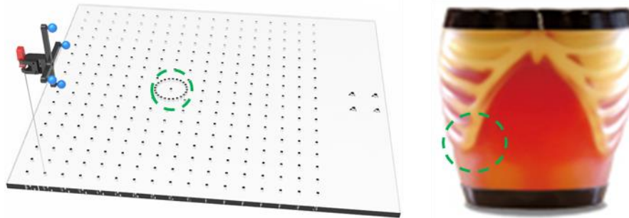
Figure 4.6. Representation of the acrylic plate (left) and abdominal phantom (right).
