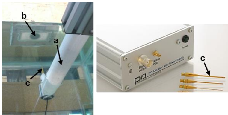
Figure 6.12. Mapping setup: a) 3D robotic arm; b) UT outside the water tank; c) needle hydrophone.
